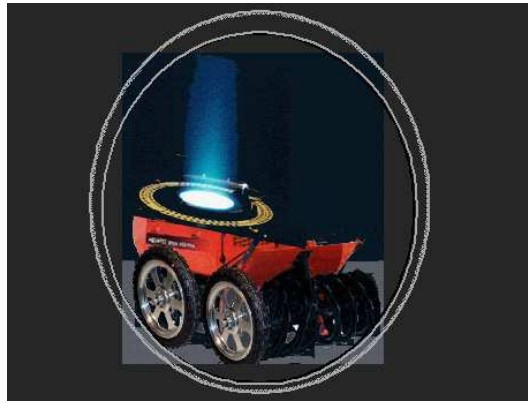
Fig. 1 The multi-layer oval envelope that will be inflated around the screw-engine at the landing time, offering a safe bouncing, rolling and a final standing up on the asteroid soil. The egg-like bag, possibly made by twin-vertical slice component, will be safely abandoned on the ground or deflated on the engine sides.
