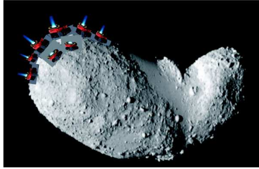
Fig. 3 A non rotating or a spinning asteroid in axis toward the Earth, may offer the simplest solution of a clustering of a few screw-engine in a well defined area, as described in figure. In principle it may exist just a point on the surface, connecting a line from the Earth toward the asteroid center of mass intersecting the body surface; however, even in the most optimistic configuration, this point by slow orbital spin will define at best a small area where to locate the engines.
